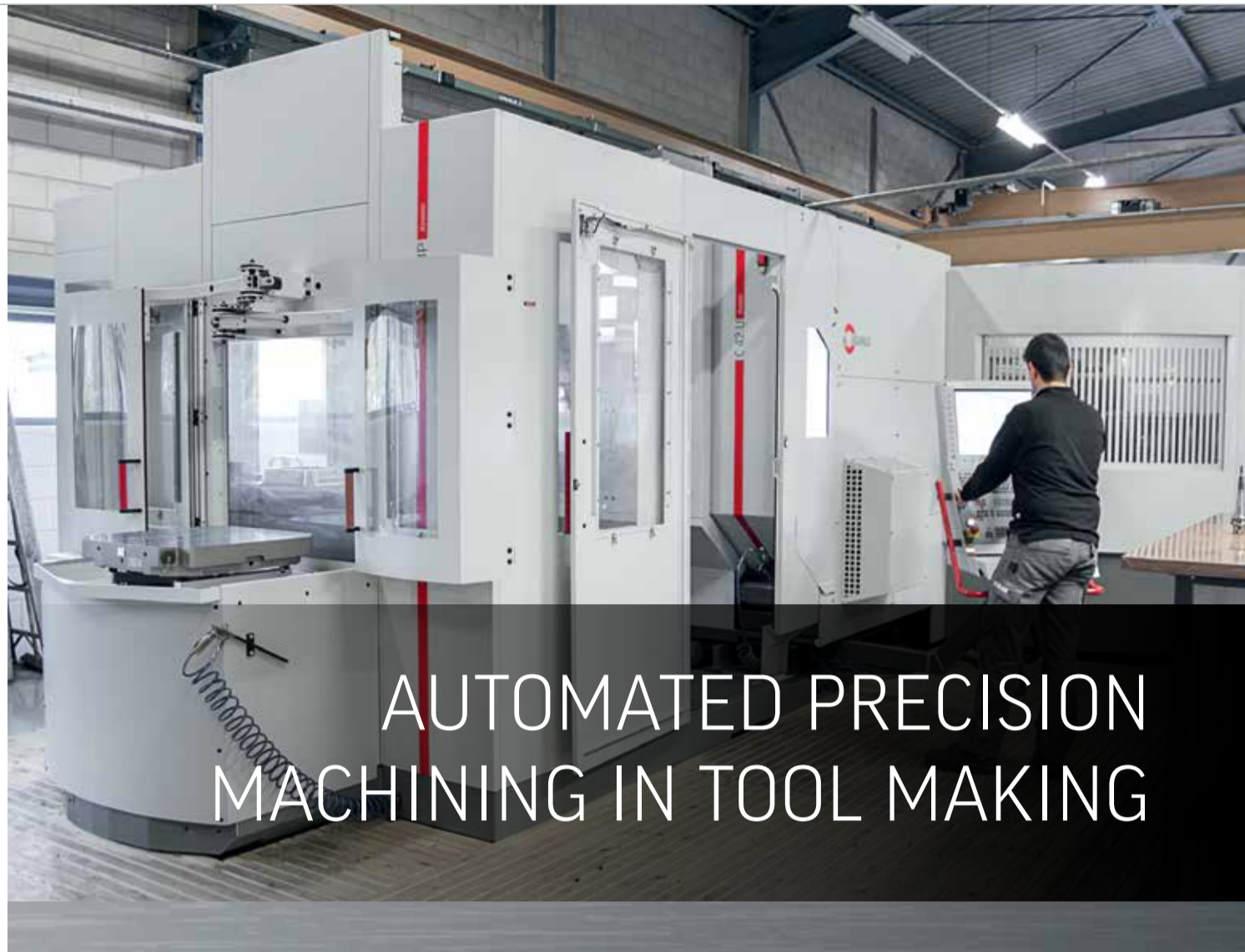
Working range of the compact 5-axis C 42 UP machining centre with the NC swivelling rotary table 800 x 630 mm for holding differently stocked pallets. On the left there is a pallet stored in the magazine pocket
