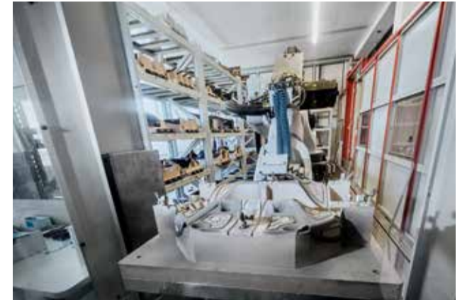
Loading/unloading (complete with workpiece clamping device and workpiece) of a loaded workpiece pallet into or out of the setup station
