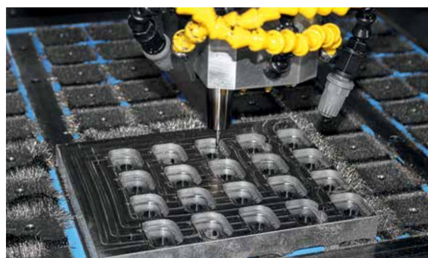
A change-pallet with assembled magnetic clamping plate and the multi-tool insert (20x) of a die cast tool system in finish machining
